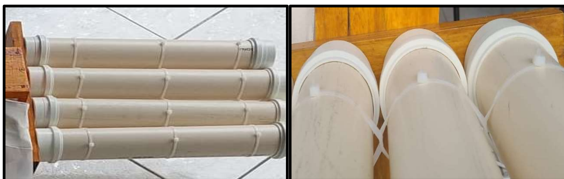
Figure 5: Side view of the PVC buoyancy system and attachment with interlaced clamps for added strength.
