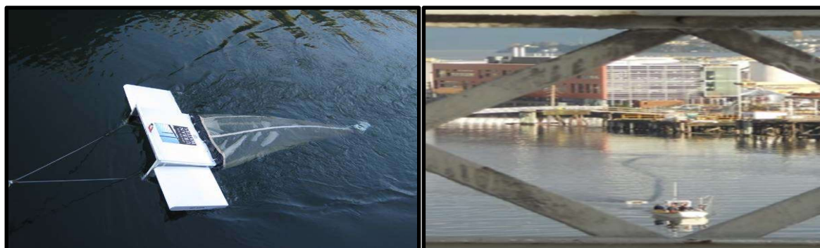
Figure 2: Floating sampler attached to a Neuston net coupled to a trailer (boat) in waters.
