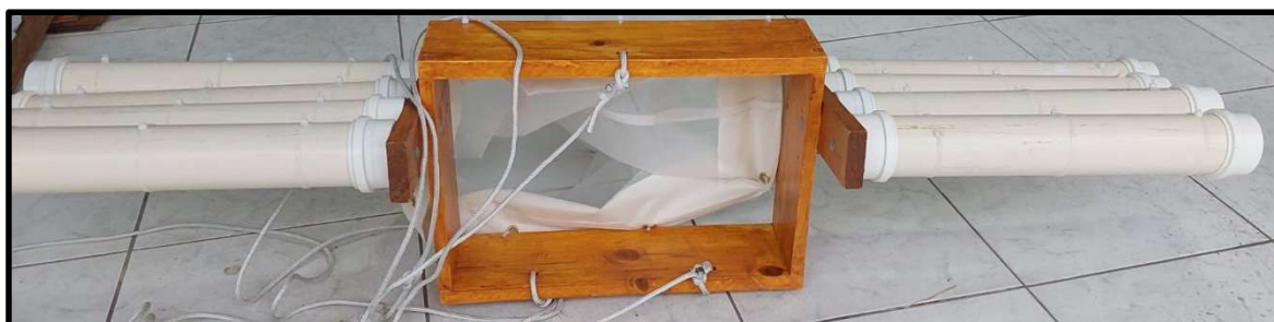
Figure 4: Front view of the Low-Cost Microplastic Net made of wood treated with marine varnish coupled with a Neuston net and PVC pipes responsible for buoyancy.
