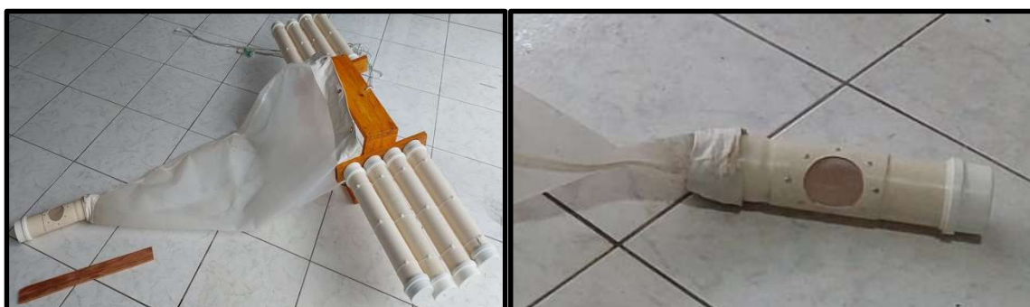
Figure 3: Low-cost Net for Microplastics and the collecting cup attached to the net.
